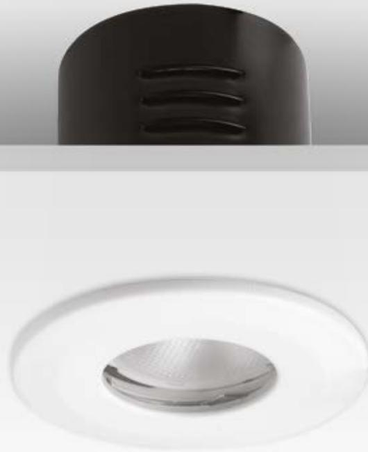
MEGAMAN® VERSOFIT provides fire protection that protects the integrity of the ceiling and prevents the spread of fire and smoke into the room above. MEGAMAN® VERSOFIT is compliant to BS476 Part 21 and is designed to withstand fire for up to 90 minutes when mounted in a timber and plaster board fire rated ceiling construction.
