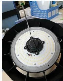
Step4: Loosen the sensor holder screw
