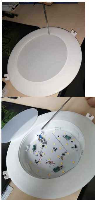
Step 1: Remove the diffuser
