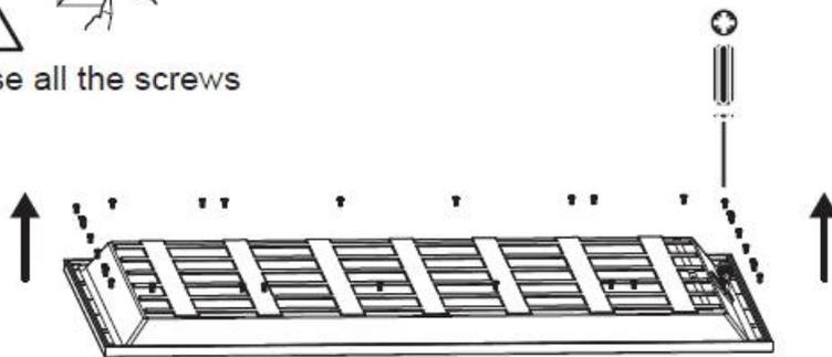
3. Disassemble the panel
