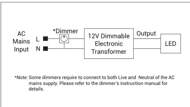
Single Dimmer and Multiple 12V Dimmable Electronic Transformer Single Lamp Connection
