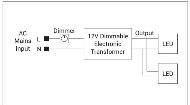
12V Dimmable Electronic Transformer Single Lamp Connection
