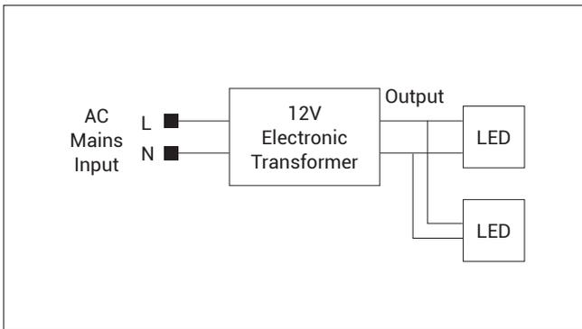
12V Dimmable Electronic Transformer Multiple Lamp Connection
