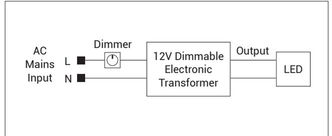
12V Electronic Transformer Multiple Lamp Connection
