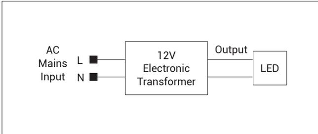
12V Dimmable Electronic Transformer Single Lamp Connection
